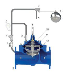
lic circuit. The needle valve (2) regulates the flow in and out of the chamber (10) to prevent pressure surges during closing.
