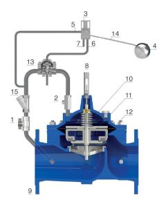
through the seat (12). The PF needle valve (2) regulates the flow in and out of the chamber to prevent pressure surges during closing.
