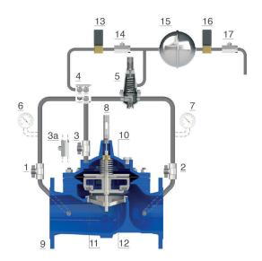
valves 14 and 17 and tank 15 increase the stability of the valve during adjustment. The flow to and from the main chamber (10) is controlled by the unique PF GR.I.F.O. (4), which makes the valve opening and closing speeds independent of each other.
