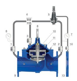
filter and three adjustable needle valves, which guarantee stability and make the valve opening and closing speeds independent.
