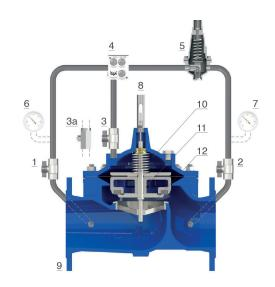
make the valve opening and closing speeds independent of each other. Thanks to the ball valves (1, 2 and 3), maintenance of the circuit and its components can also be carried out without interrupting the flow through the main valve.
