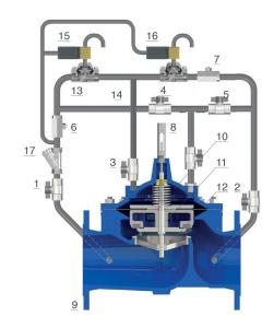
A filter (17), installed upstream, also protects the solenoid and other circuit components from contact with impurities and debris.
