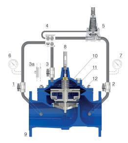
ensure stability and make the valve opening and closing speeds independent of each other.
