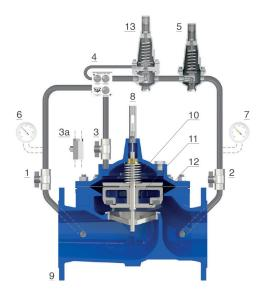
opening and closing speeds independent of each other. Thanks to the ball valves (1, 2 and 3), maintenance of the circuit and its components can also be carried out without interrupting the flow through the main valve.
