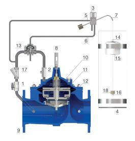
(7) downwards. This causes the pressure in the control chamber (10) to be discharged into the atmosphere, resulting in the plug (11) rising and the flow resuming through the seat (12).
