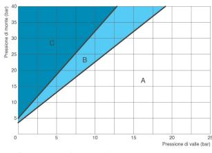
Ensure that the point corresponding to the operating condition of the valve, appropriate to the required flow rate, falls in zone A of the graph (abscissa: the downstream pressure values; ordinate: the upstream pressure values). The graph refers to valves modulating with an opening percentage of 35-40%, at standard temperature and altitude below 300 m. In pressure support, the differential must not exceed 17 bar. The relief function tolerates larger differentials.
