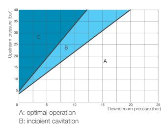
**Pressure drops chart** Ensure that the point corresponding to the operating condition of the valve appropriate to the required flow rate, identified by the values of the downstream pressure (in abscissa) and upstream pressure (in ordinate), falls in zone A in the graph.
