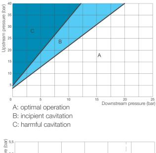
**Pressure drops chart** Ensure that the point corresponding to the operating condition of the valve appropriate to the required flow rate, identified by the values of the downstream pressure (in abscissa) and upstream pressure (in ordinate), falls in zone A in the graph.
