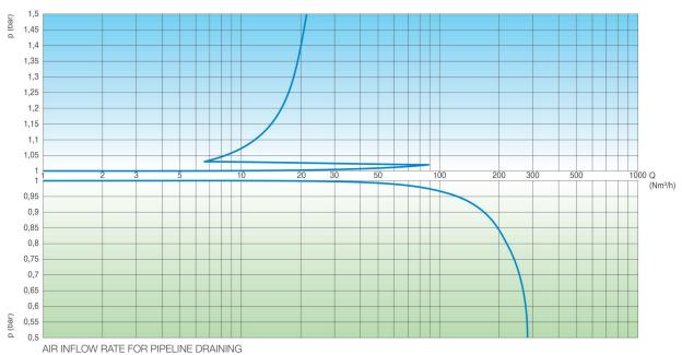
Air flow charts are obtained in Kg/s from laboratory tests and numerical analysis, without filtering, and converted to Nm/h by applying a safety factor.
