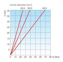
AIR FLOW RATE DURING DEGASSING
