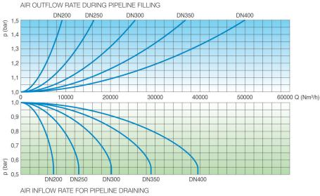
Air flow charts are obtained in Kg/s from laboratory tests and numerical analysis, without filtering, and converted to Nm3/h by applying an appropriate safety factor.
