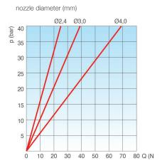
AIR FLOW RATE DURING DEGASSING
