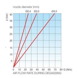
Air flow charts are obtained in Kg/s from laboratory tests and numerical analysis, without filtering, and converted to Nm3/h by applying an appropriate safety factor.
