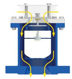
• Very easy to intervene from above without removing the air valve from the pipeline.
