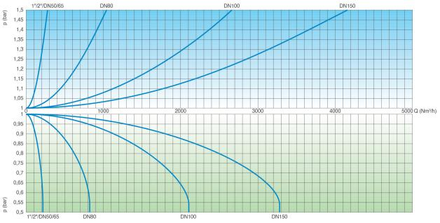
AIR OUTFLOW RATE FOR PIPELINE DRAINING
