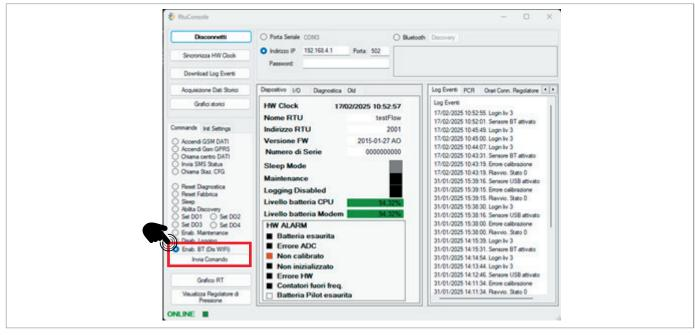
Fig. 5.12. Rainbow interface for switching to Bluetooth mode
