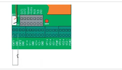
Fig. 4.5. Digital input terminal block
