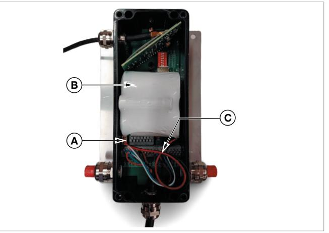
Replacing the battery pack
