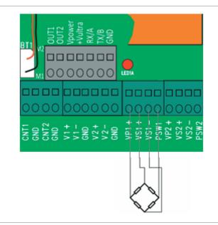
Fig. 4.4. Pressure input terminal block
