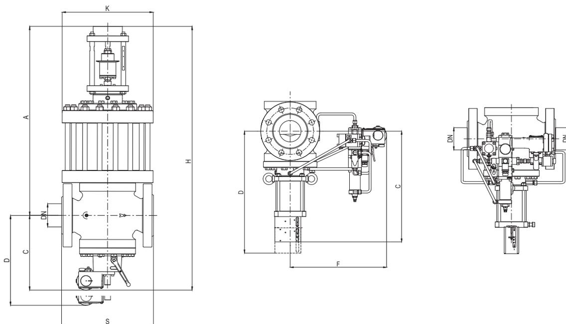
**Figura 12** Dimensiones Syncroflux + DB/819 + SB/82 o HB/97
