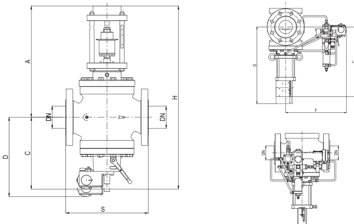
**Figura 10** Syncroflux + dimensiones SB/82 o HB/97
