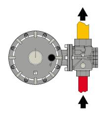
Figure 6 Dival 500 vertical installation 1
