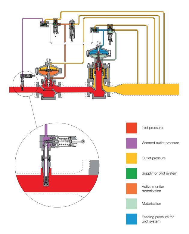
Figure 4 ATF 15 typical installation
