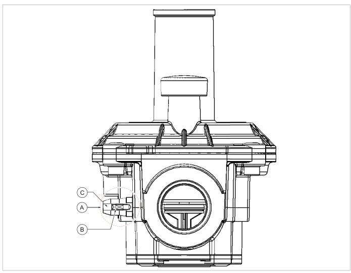
Fig. 4.11. Using standard pressure tap
