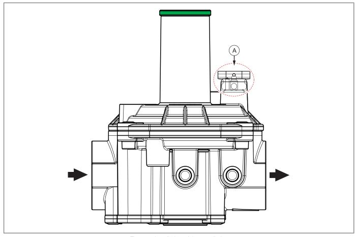
Fig. 4.9. Installation of the vent limiter
