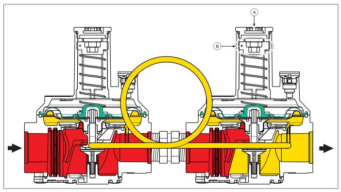
Fig. 7.24. Operating pressure adjustment (Standard version)
