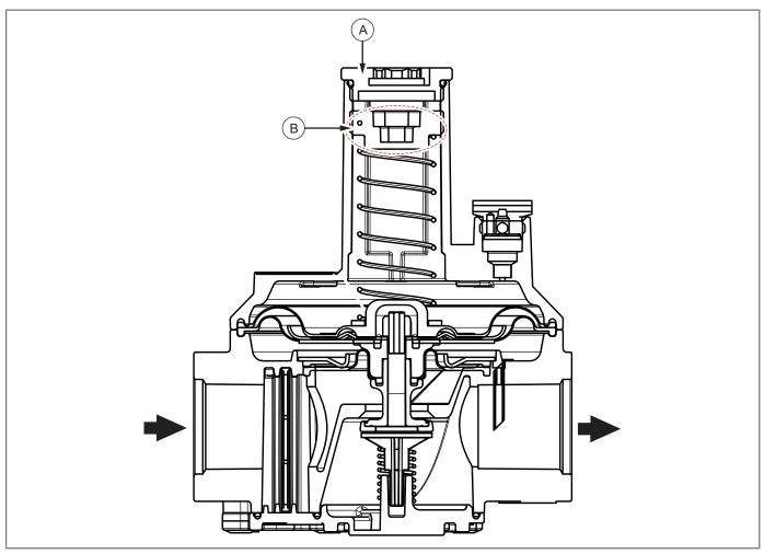
Fig. 7.21. Operating pressure adjustment (Standard version)
