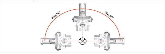
Fig. 7.16. Correct mounting position of the Standard/Goval versions
