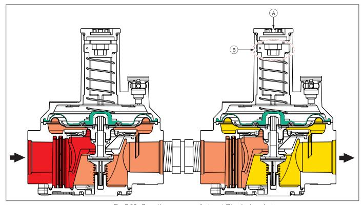
Fig. 7.25. Operating pressure adjustment (Standard version)
