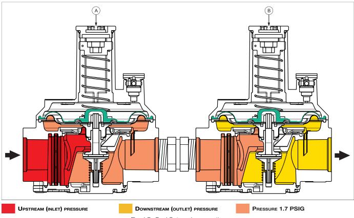
Fig. 4.7. Dual Cut version operation
