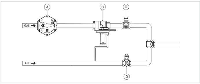
Fig. 7.19. Ratio version installation examples
