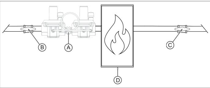
Fig. 7.20. Example of installation of the OPD/Dual Cut versions
