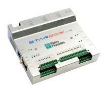
**Starbox LX2** embodies the typical characteristics of a data logger with advanced multimedia features. In fact, it is a system where process control, multimedia capabilities, remote management and the internet are available and usable with identical operating standards and can be activated in a simple and intuitive way.
