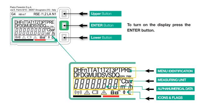
An all-segment lit-up test is performed for a couple of seconds upon display activation, then the Current Index of Converted Volume is shown in cubic meters [m3] with 5 units and 3 decimals.
