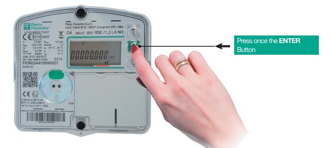
\* Example of the Display activation and visualization of the Current Index of Converted Volume [m3] – Icon T
