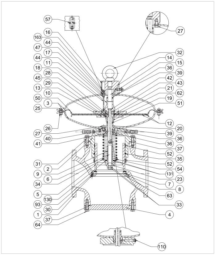
Fig. 9.71. Regulator REVAL 182 DN 6" to 8"
