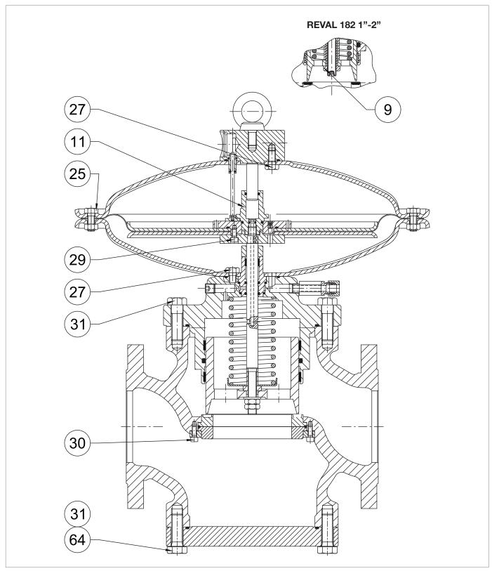
Fig. 9.46. Tightening torques REVAL 182
