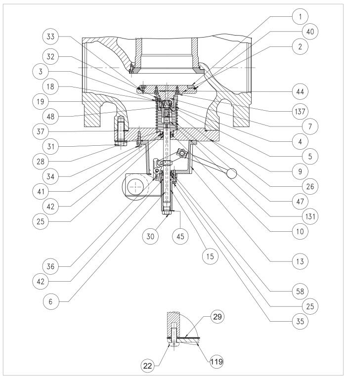
Built-in slam-shut valve SB/82 DN 4" - 8"
