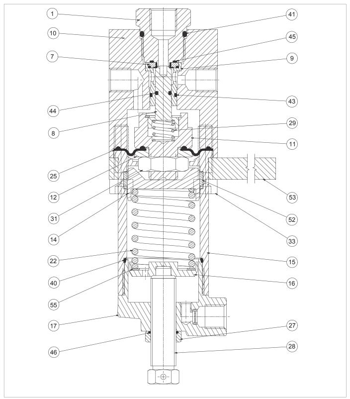
Fig. 9.86. M/A accelerating valve
