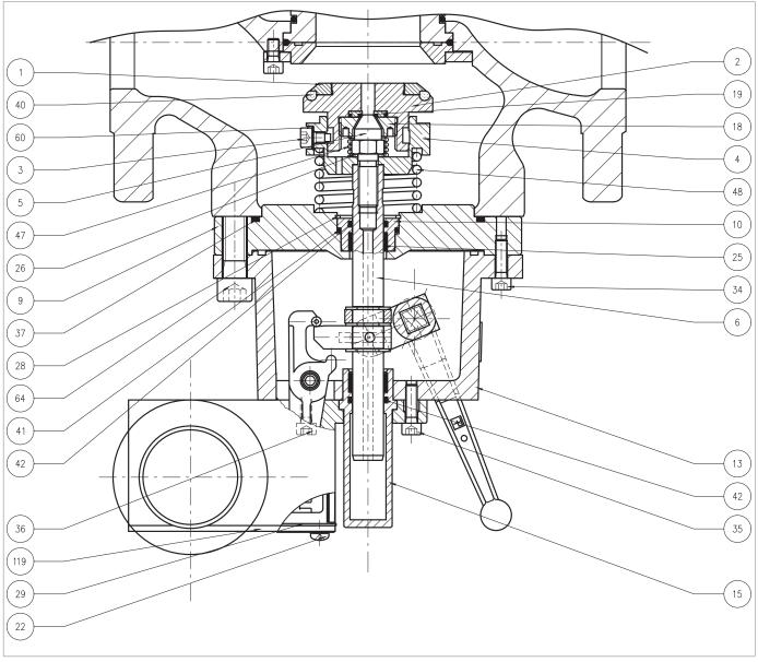
Fig. 9.93. Built-in slam-shut valve SB/82 DN 2"- 3"
