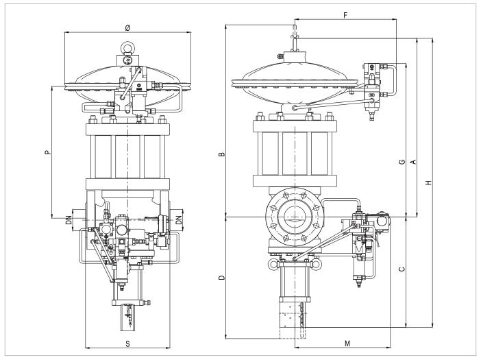
Fig. 5.24. Physical characteristics REVAL 182 + DB/182 + HB/97
