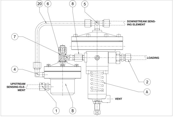
Fig. 9.83. Pilot 201/A and pre-regulator R31/A
