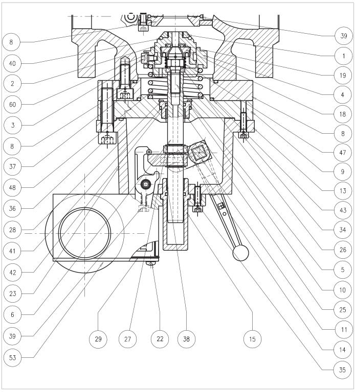
Built-in slam-shut valve SB/82 DN 1"
