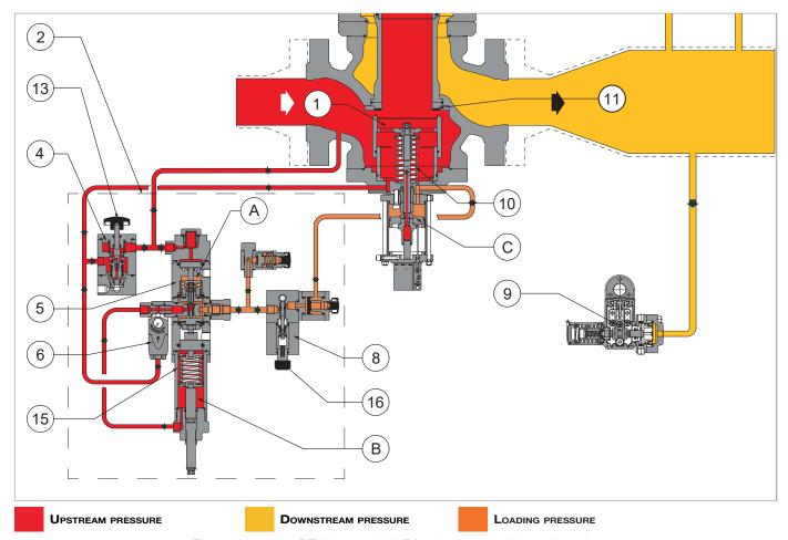
Fig. 4.13. REVAL 182 with HB/97 incorporated slam-shut valve
