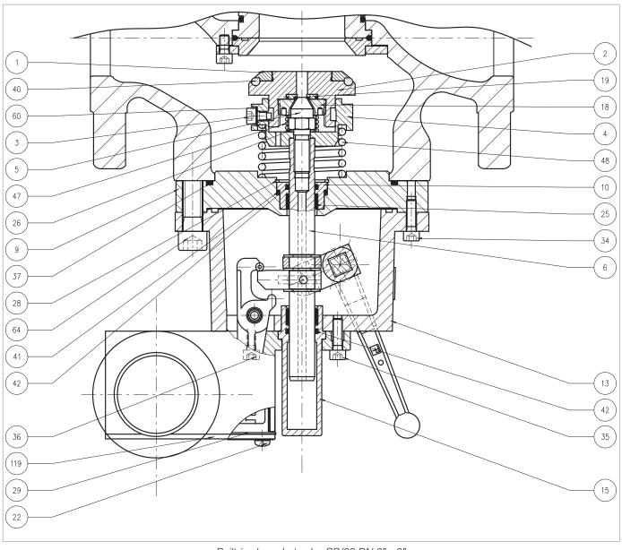
Built-in slam-shut valve SB/82 DN 2" - 3"
