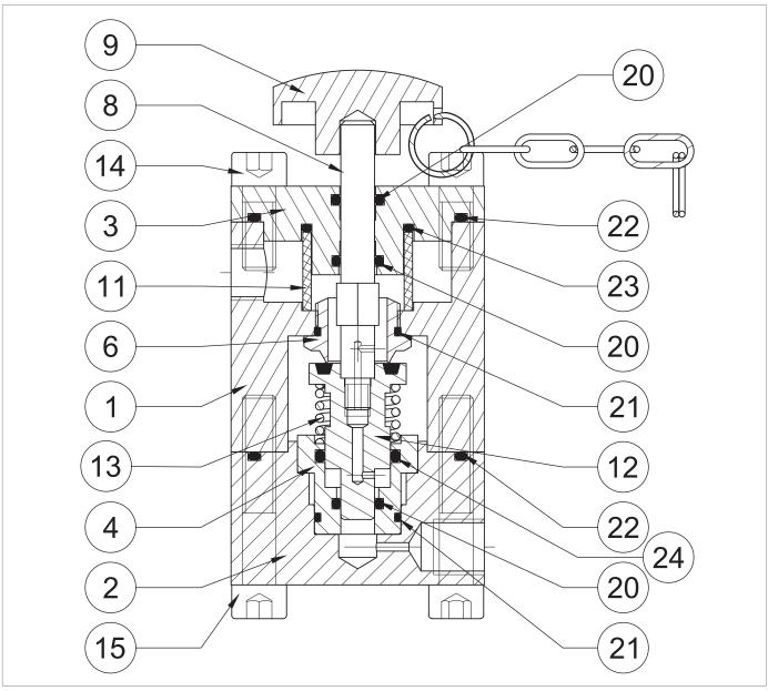
Fig. 9.101. HP2/2 bypass device
