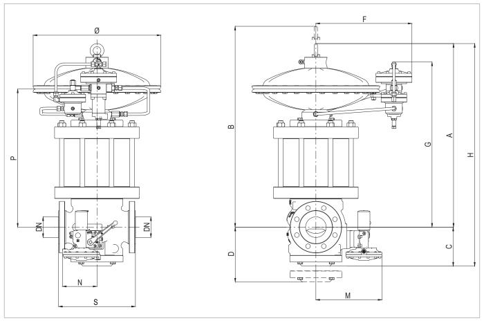
Fig. 5.22. Physical characteristics REVAL 182 + DB/182 + SA
