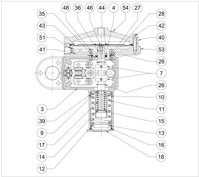
Fig. 9.96. Pressure switch Mod. 101M/101MH
