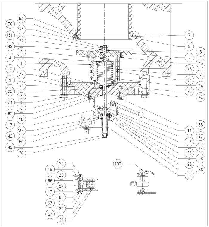
Fig. 9.95. Built-in slam-shut valve SB/82 DN 10"
