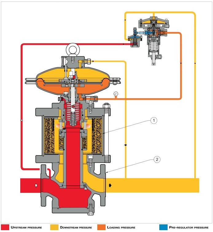
Fig. 4.3. Built-in silencer DB/182
