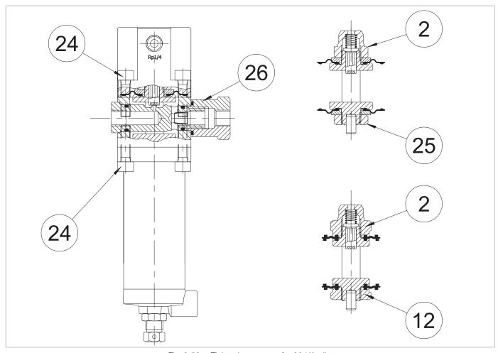
Fig. 9.50. Tightening torques for 204/A pilot
