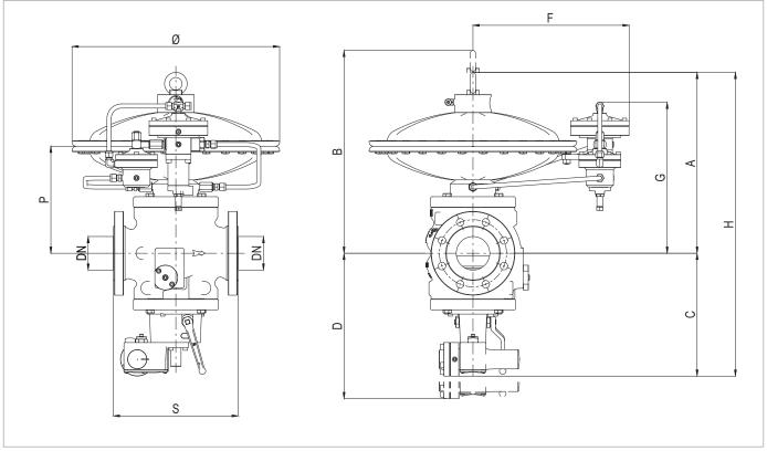
Fig. 5.19. Physical characteristics REVAL 182 + SB/82
