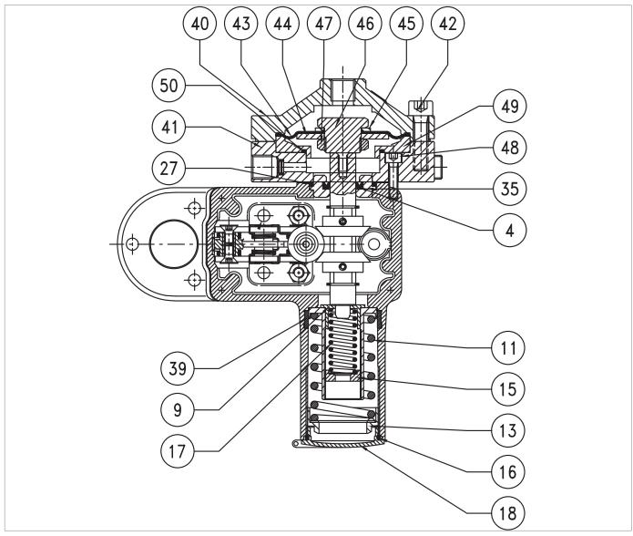
Fig. 9.97. Pressure switch Mod. 102M/102MH
