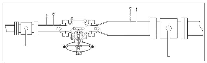
Fig. 6.28. Inverted position
