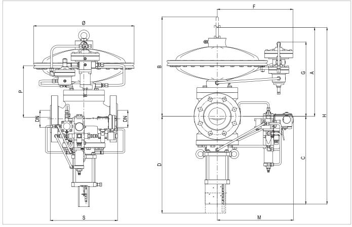
Fig. 5.20. Physical characteristics REVAL 182 + HB/97
