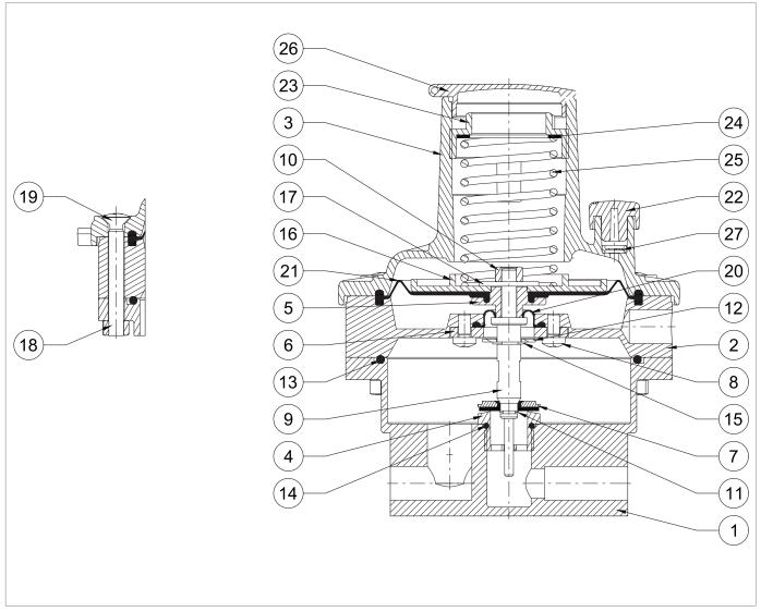
Fig. 9.85. V/25 accelerating valve
