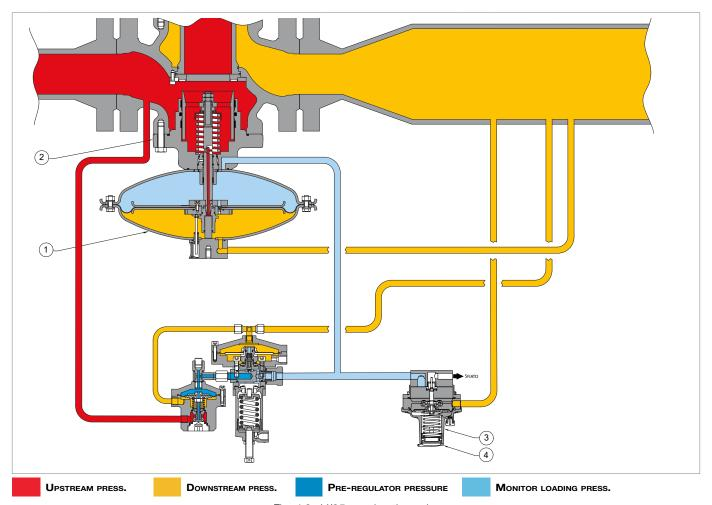
Fig. 4.9. V/25 accelerating valve
