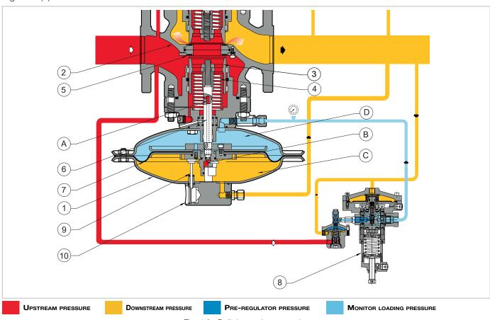
Fig. 4.6. Built-in monitor operation
