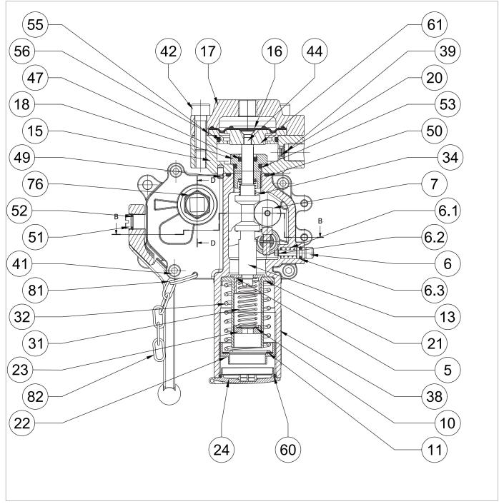
Fig. 9.90. Pressure switch SA-93
