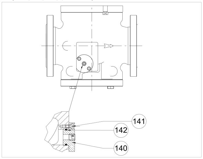
Fig. 9.68. Detail of the regulator cap
