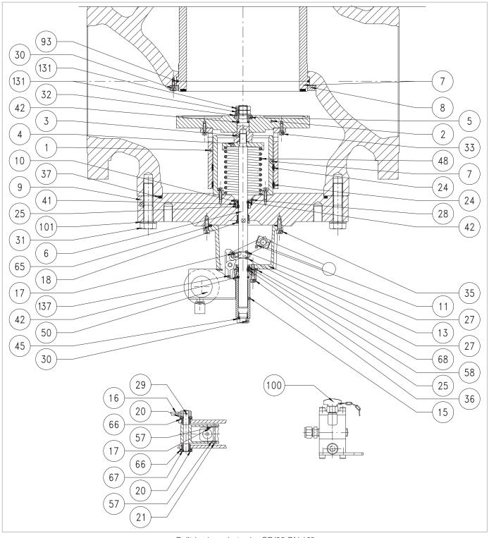
Built-in slam-shut valve SB/82 DN 10"
