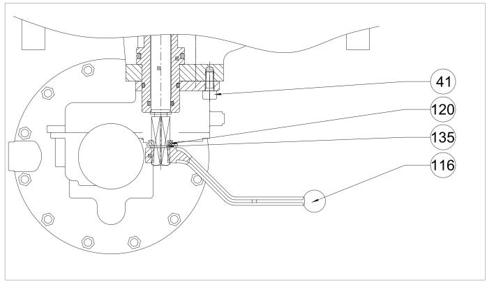
Fig. 9.91. Pressure switch mod. SA
