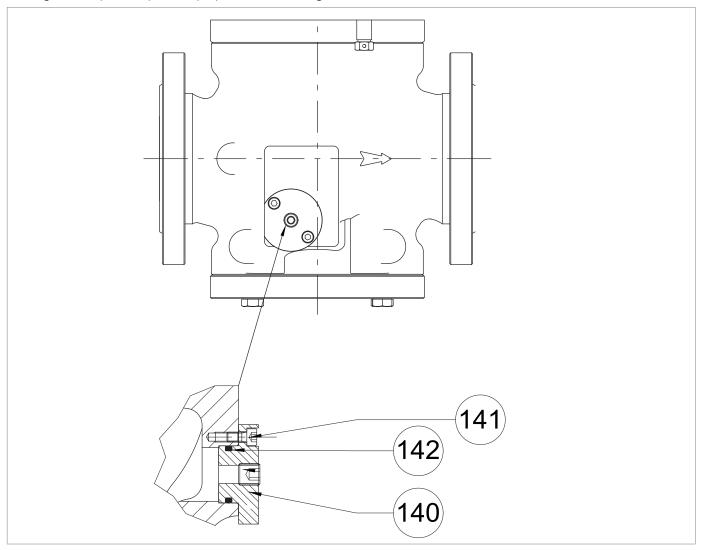
Fig. 9.70. Detail of the regulator cap
