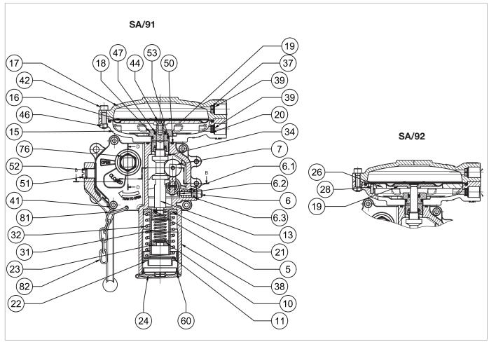
Fig. 9.89. Pressure switch SA-91, SA-92
