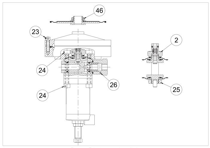
Fig. 9.49. Tightening torques for 201/A pilot
