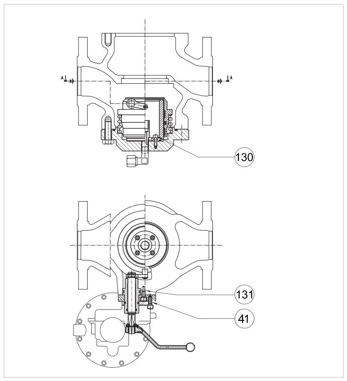
Fig. 9.53. SA slam-shut valve tightening torques
