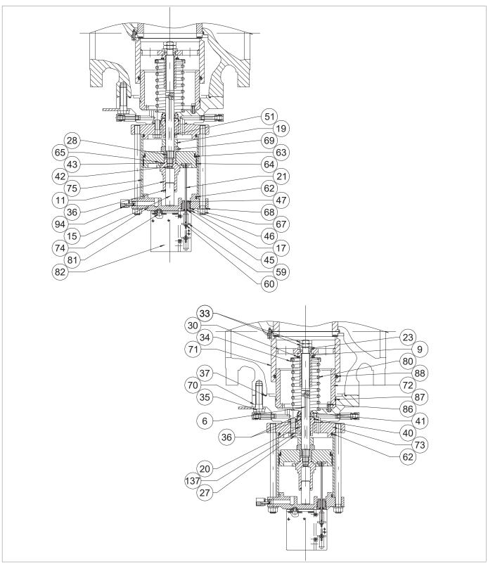
Fig. 9.100. HB/97 built-in slam-shut valve
