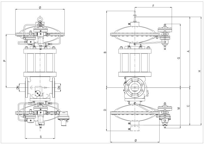
Fig. 5.21. REVAL 182 + DB/82 + PM/182 physical characteristics
