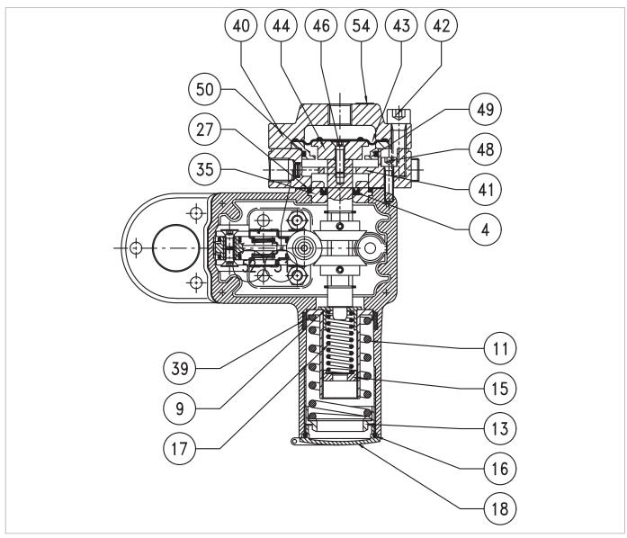
Fig. 9.98. Pressure switch Mod. 103M/103MH
