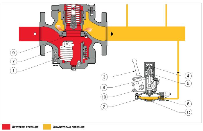
Built-in slam-shut valve SA Fig. 4.11.
