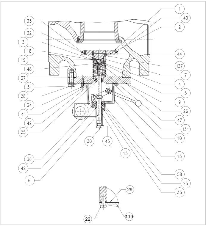
Fig. 9.94. Built-in slam-shut valve SB/82 DN 4" - 8"
