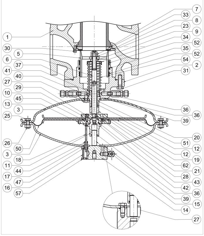
Fig. 9.75. Built-in monitor PM/182 2" ½ to 4"
