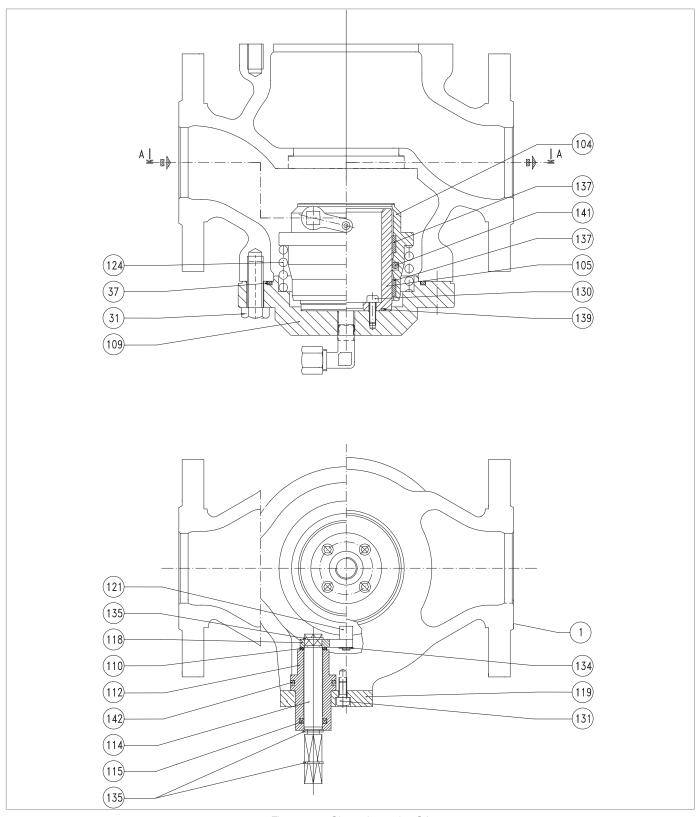
Fig. 9.87. Slam-shut valve SA
