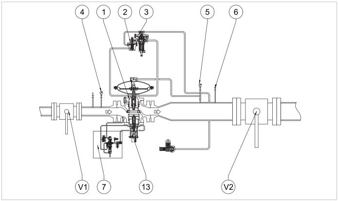
Fig. 8.40. Sealing of the HB/ 97 slam-shut valve during shut-off
