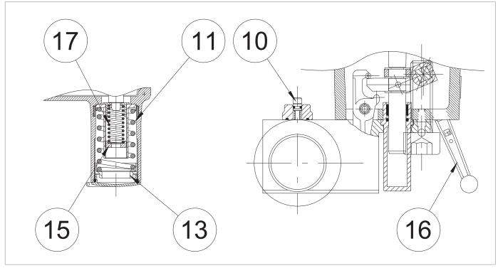
Fig. 8.44. Calibration of pressure switches mod. 100
