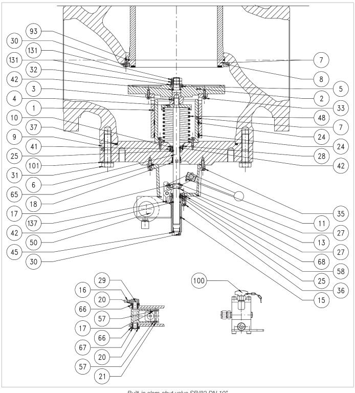
Built-in slam-shut valve SB/82 DN 10"
