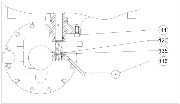
Fig. 9.88. Pressure switch mod. SA
