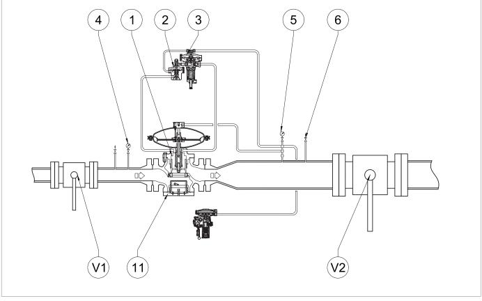
Fig. 8.36. Commissioning of the regulator REVAL 182 with SA slam-shut valve
