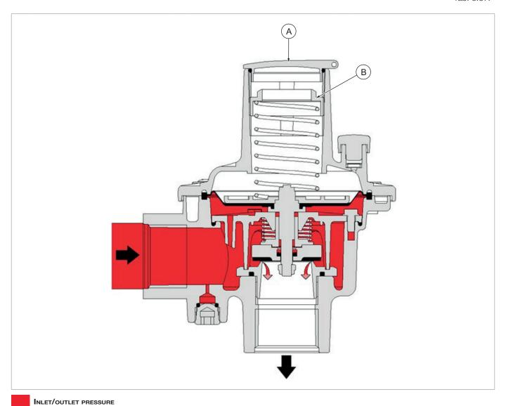
Fig. 8.8. Adjustments VS/AM 65
