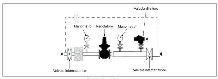
Fig. 6.5. Installation scheme
