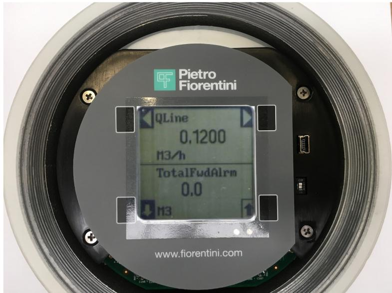
Figure 6-1 - LCD and keypad (front cover removed)
