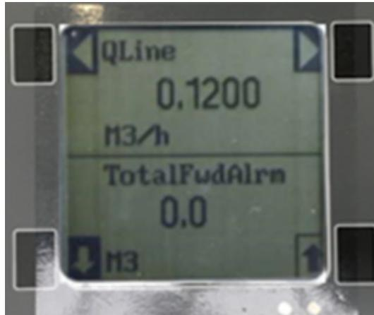
The upper display is “static” - that is only the selected parameter is displayed. The parameter may be changed manually using the ◀ <left> and ▶ <right> scroll keys. The lower display will automatically scroll through the remaining parameters. The full list of parameters is shown below.
