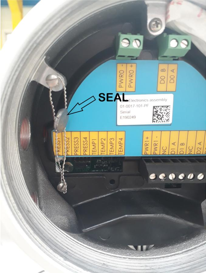
**Figure 2-2: Electronic assembly and transducer connector cover seal**
