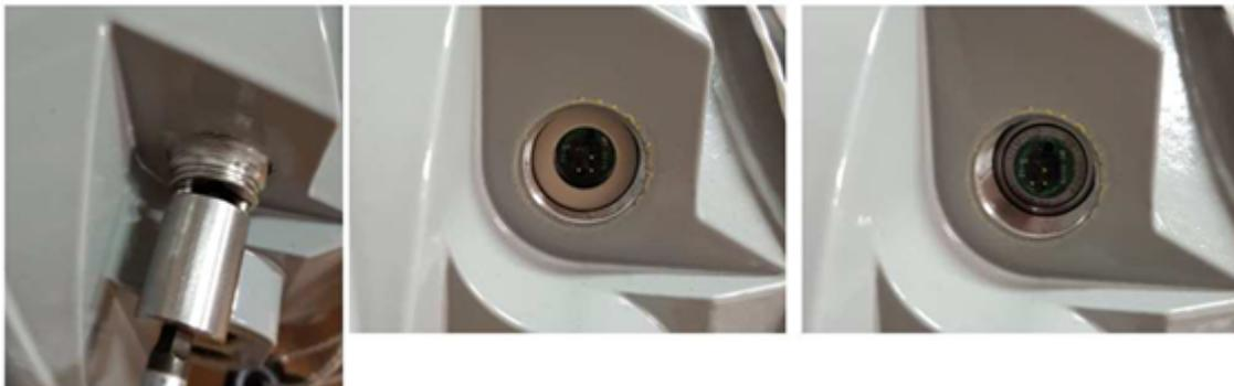
8. Now using a flat nose plier grab one of the connector pins and gently pull out the transducer. Be careful not to bend the pin, pull straight along the axis of the transducer port. Below picture shows the transducer removed.
