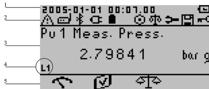
**Figure 29 Common structure of the pages**
