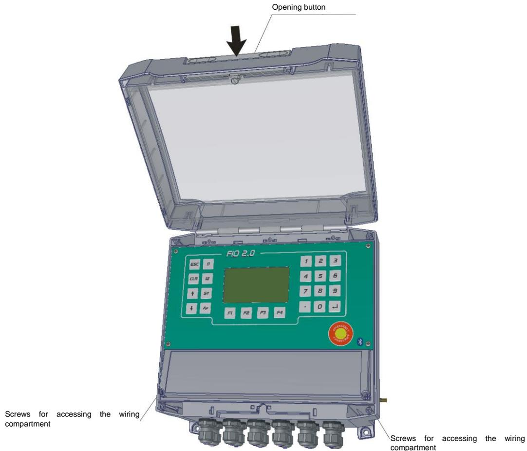
**Figure 21 Access to the wiring compartment**
