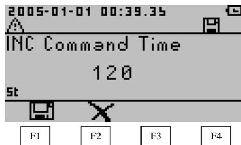
**Figure 31 Saving the configuration**
