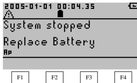
**Figure 45 Stopped system: replace the battery**
