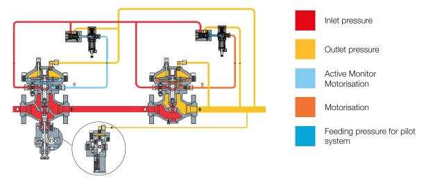
Figure 5 Dixi AP with In-line monitor setup
