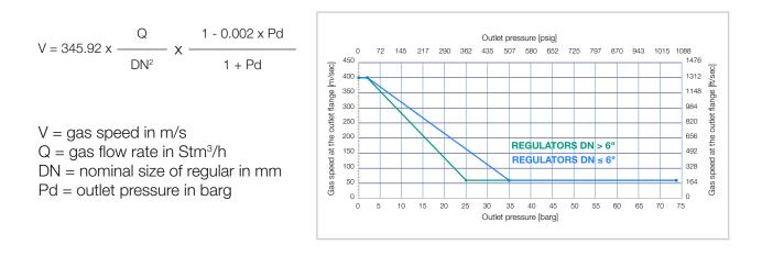
Sizing of regulators is usually made based on valve Cg value (table 8).
