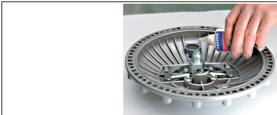
Adhesive application for anti-pumping valve:
