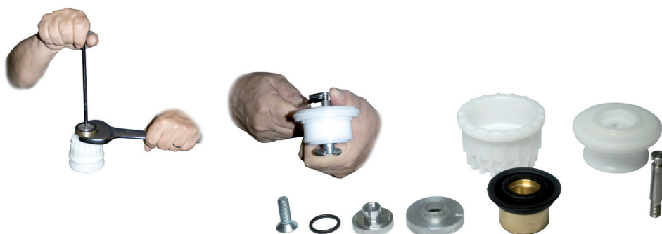
Balancing group disassembling :
