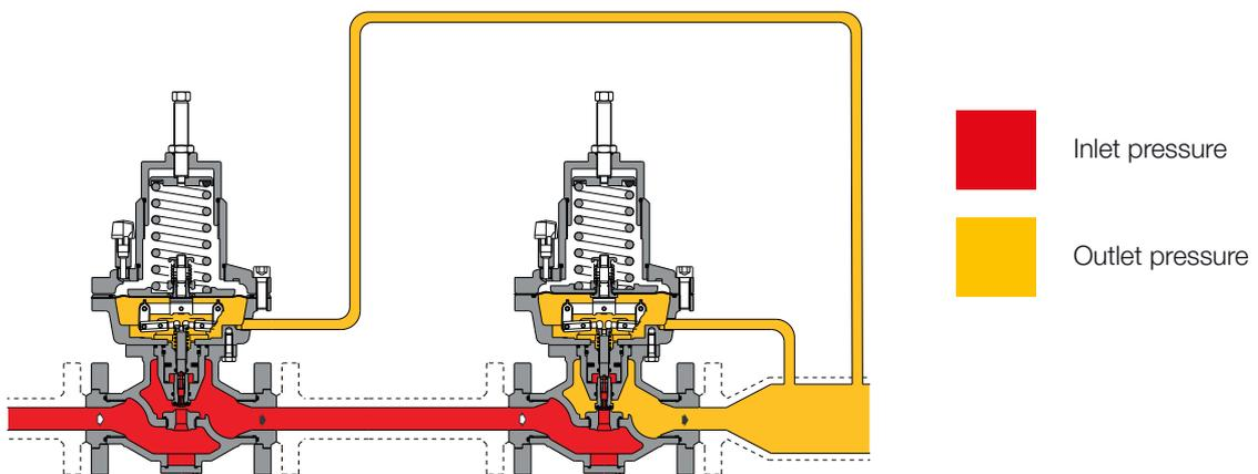
**Figure 5** Dival 160 AP with In-line monitor setup
