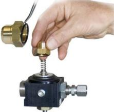
12) Remove the obturator together with the spring and the diaphragm
