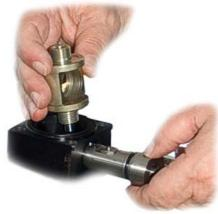
20) Unscrew the valve seat from the valve seat group
