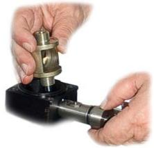
16) Unscrew the valve seat from valve seat group
