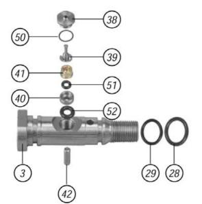
(3) valve seat group, (38) valve seat,(39) modular piston,(40) guide,(41) connector, (42) cylindrical pin. (28-29-50-51-52) O-ring
