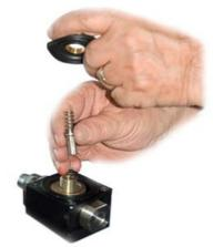
13) Remove the valve seat group fitting
