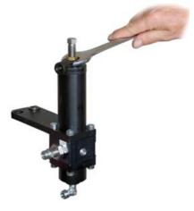
3) Remove the cap together with the spring and the spring guide
