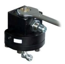
7) Remove the nut together with the disc and the diaphragm
