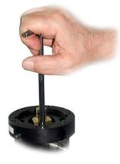
13) Remove the flange from the valve body
