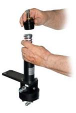
4) Unscrew and remove the fixing bolts of the muff to the body
