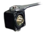
19) Separate the valve seat group from the valve body and the diaphragm support
