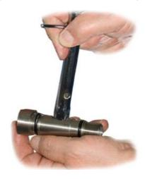
17) Remove the valve seat and the inside components
