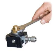
11) Remove the obturator support together with the spring and remove the o-ring
