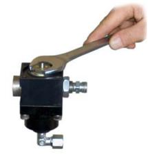
7) Remove the nut together with the disc and the diaphragm
