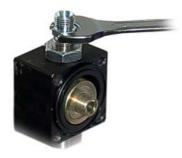
14) Unscrew and remove the fixing nut of the valve seat group to the valve body
