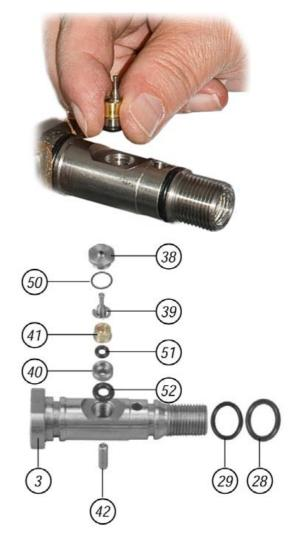
(3) valve seat group, (38) valve seat,(39) modular piston,(40) guide,(41) connector, (42) cylindrical pin. (28-29-50-51-52) O-ring
