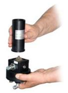
6) Unscrew the fixing nut
