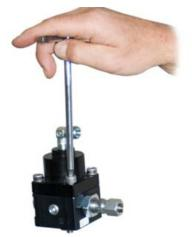
9) Remove the head cap together with the spring
