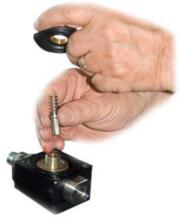
17) Remove the valve seat group fitting
