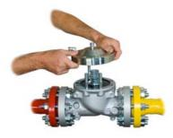
5) Take out the diaphragm group and separate the single parts (3 - 9 and 11)
