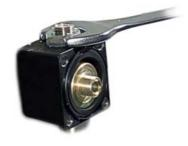
15) Separate the valve seat group from the valve body and the diaphragm support
