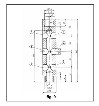
1 and 2 Connect to regulators heads 3 and 4 Connect to pilots
