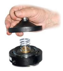
10) Remove the spring and the diaphragm
