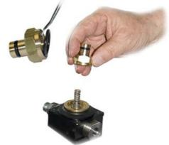
16) Remove the obturator together with the spring and the diaphragm
